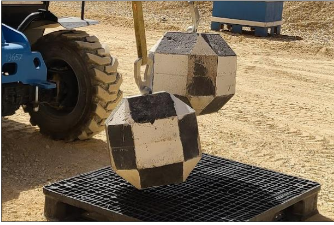
Figure 3. R1-type synthetic rhombicuboctahedron-shaped rocks.
