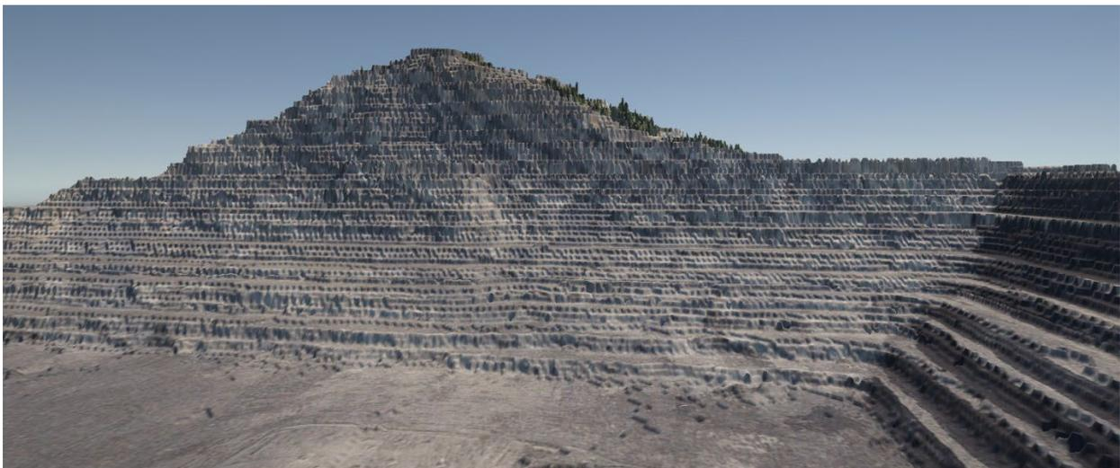
Figure 4-8. 3D model of Mine 7 pit slope generated in Unity from a digital elevation map (DEM) file
