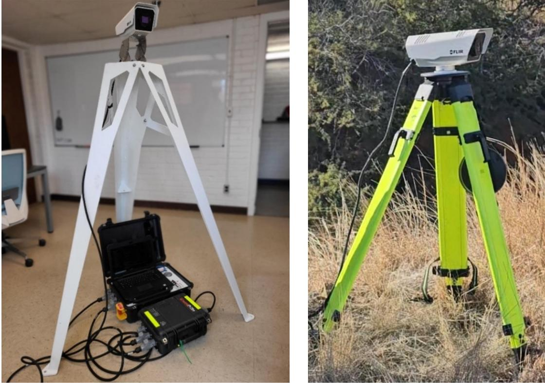
Figure 5-3. Prototype tactical system tripod options: *(left)* heavy-duty tripod option, shown with prototype system camera, processing unit, and PoE system in an office environment; *(right)* lightweight tripod option, shown with thermal camera (remainder of standalone system not visible), shown during a deployment test.
