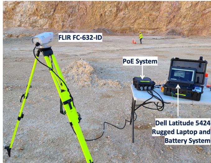
Figure 5-1. Prototype tactical monitoring system deployed with Tripod 2 at a mine in Nevada.
