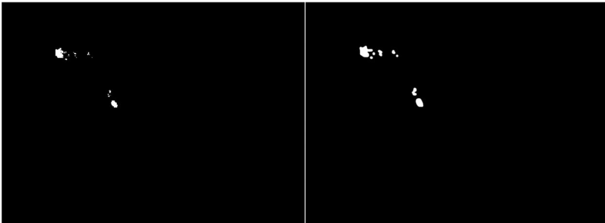
Figure A-3. Motion Region Refinement. The left frame represents the areas of motion identified in the right frame of Figure A-2 above. The right frame shows these regions after the dilation and contraction process, consolidating nearby movements.
