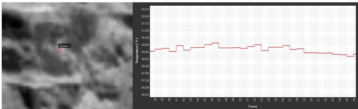
Figure A-1. Depiction of Thermal Video Noise. The left frame shows a detail of a radiometric thermal video taken with the FLIR A400 scientific thermal camera, with a single pixel highlighted. The right frame shows the temperature change of this pixel over 29 frames, representing approximately 2 seconds of elapsed time.
