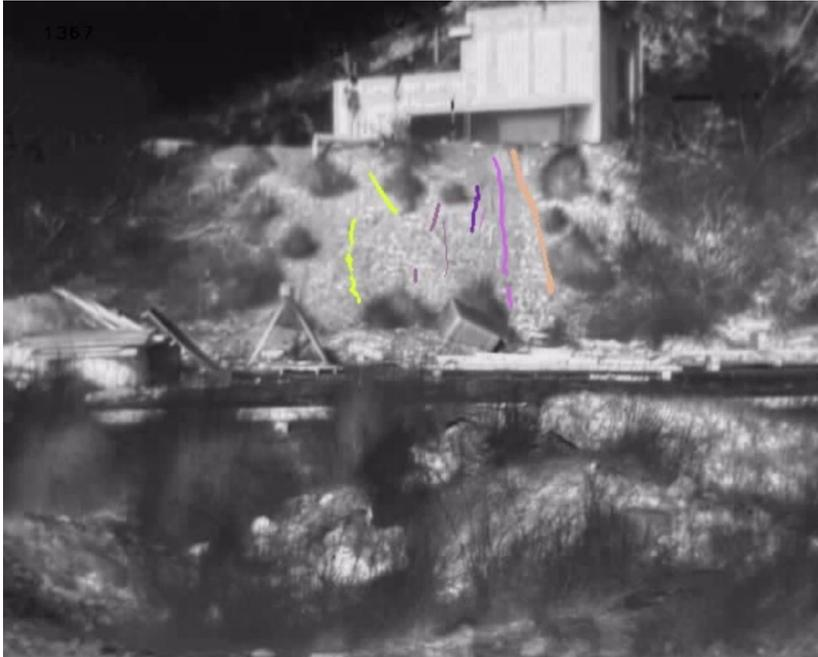
Figure 4-4. Still image depicting multiple rockfall traces from a test of the prototype tactical system at the SX Mine. Each color overlaying the grayscale background indicates a separate fall event (some of which include a secondary fall representing dislodged material). Line thickness varies based on the amount of moving material observed.
