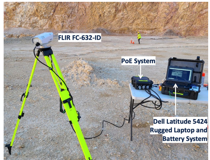
Fig. 1. Prototype tactical monitoring system deployed at a mine in Nevada.
