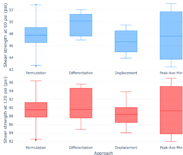
Fig 11. Box and Whisker plots of shear strength ( \tau ) calculated at 60 psi normal (above) and 120 psi normal (below) stresses.
