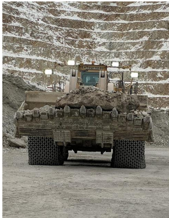
Figure 2. Mine loader carrying a boulder to be dropped for synthetic rockfall test.
