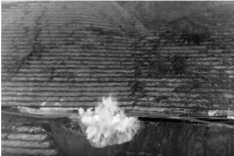
Figure 5. CAM2 thermal imagery capture of a blast event.
