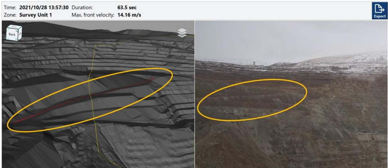
Figure 11. RockSpot Doppler radar "unwanted" detection of a haul truck driving on a haulage ramp.
